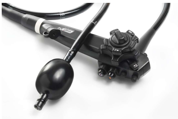
Figure 4 Newly introduced G-EYE endoscope is equipped with a balloon at the distal bending section of the endoscope. During withdrawal the balloon is inflated thereby stabilizing the endoscope for subsequent therapeutic maneuvers. In addition the balloon yields in a straightening of the colonic folds thereby potentially improving adenoma detection rates (Image with kind permission from Smart Medical).
